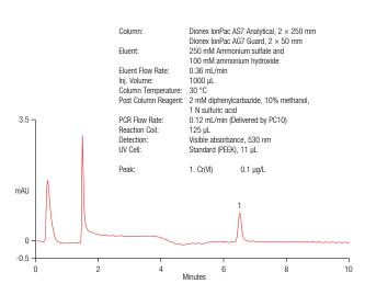
Figure 1. Determination of Cr(VI) in HIW using a Dionex Integrion HPIC system.
