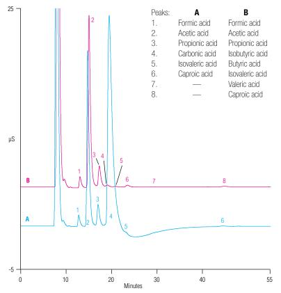
Overlay of chromatograms of spiked wastewater with and without a Dionex CRD 200 device installed.
