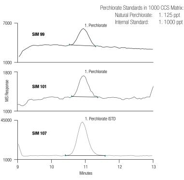
High ionic matrix spiked with 125 ppt perchlorate and internal standard.
