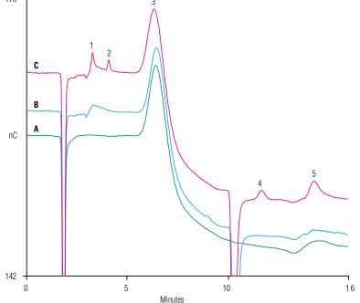
Comparison of 1:10 dilution of City A municipal wastewater effluent B) without and C) with chelates added.
