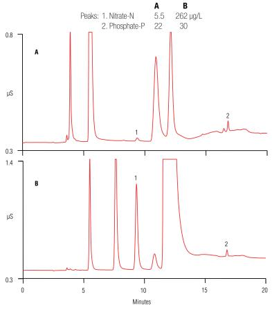
Comparison between (A) undigested and (B) digested raw sewage water.
