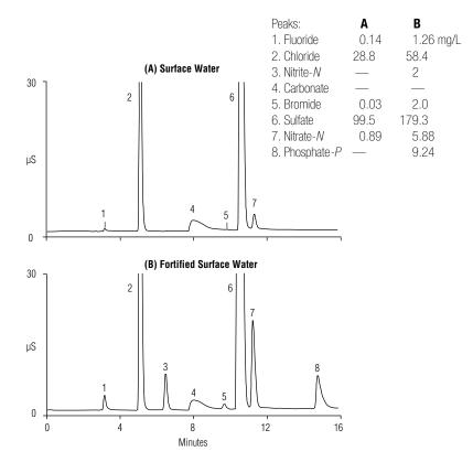
Determination of inorganic anions in (A) surface water and (B) fortified surface water using the Dionex IonPac AS18 column.
