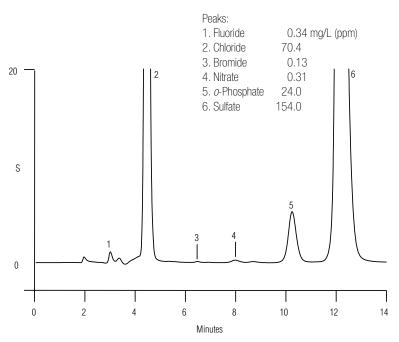
Determination of inorganic anions in domestic wastewater using a Dionex IonPac AS14 column.
