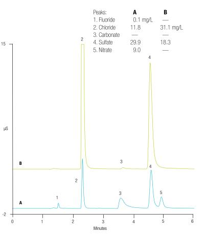
Fast anion determinations of the Salton Sea area water samples using high-pressure IC.
