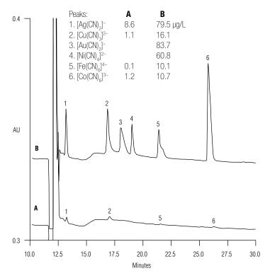
Anion-exchange separation with preconcentration and absorbance detection at 215 nm of metal cyanide complexes in drinking water from a municipal well. Drinking water matrix blank (A) and matrix spiked with metal cyanide complexes (B).
