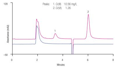
Overlay of the chromatograms of the wastewater sample and the sampled spiked with 10 mg/L Cr(III) and 0.5 mg/L Cr(VI).
