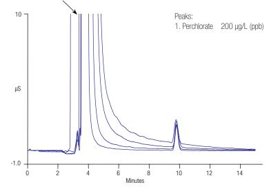
Effect of sulfate on perchlorate recovery on the Dionex IonPac AS16 column.
