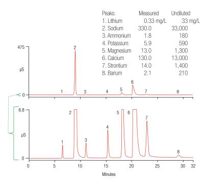
Determination of cations in fracturing flowback water (F4) using a standard bore column.
