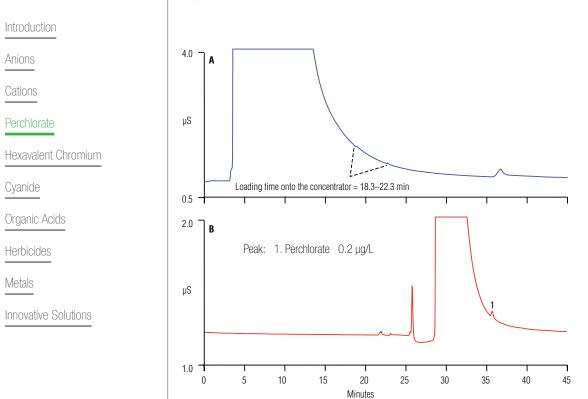
Chromatograms of synthetic high inorganic water containing 1000 mg/L each of chloride, sulfate, and bicarbonate fortified with 0.2  $\mu$ g/L perchlorate in (A) first dimension and (B) second dimension.
