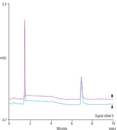
Determination of chromate (0.1 µg/L) in A) DI water and B) HIW on a Dionex ICS-2100 system. Postcolumn reagent delivered by an AXP pump. Flow cell: semi-micro (PEEK).
