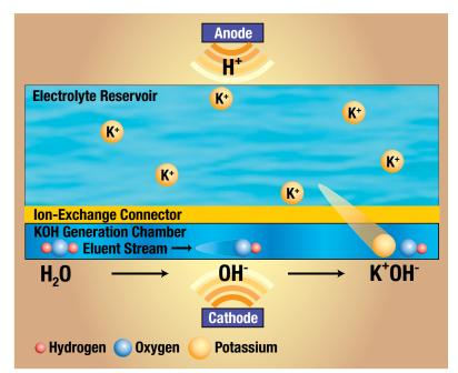
The Dionex EGC III KOH cartridge consists of a KOH generation chamber and a K<sup>+</sup> electrolyte reservoir, connected by a cation exchange connector. A high-pressure connector permits the passage of K<sup>+</sup> ions from the K<sup>+</sup> electrolyte reservoir into the electroytic chamber.
