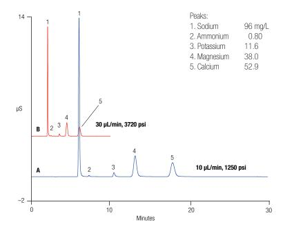
Fast, high-pressure cation separations in a wastewater sample using high-pressure capillary IC.
