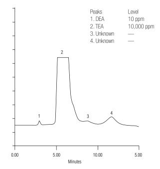
Diethanolamine determination in an oil refinery triethanolamine scrubber solution.
