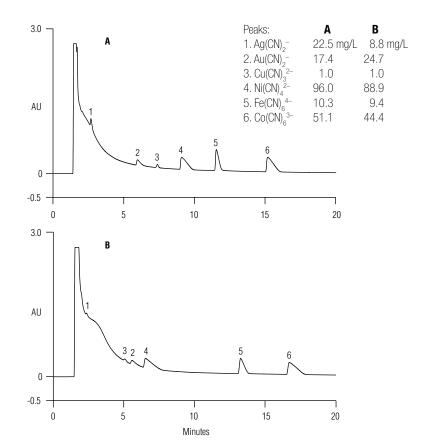
Determination of metal cyanide complexes in wastewater from a former manufactured gas plant.
