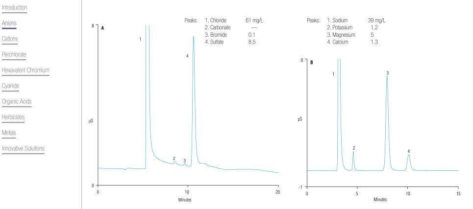
San Francisco, CA bay water: determination of common (A) inorganic anions using the Dionex IonPac AS18 column and (B) cations using the Dionex IonPac CS12A column.
