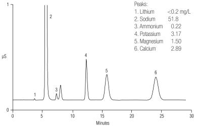
Determination of inorganic cations and ammonium in industrial wastewater with the Dionex IonPac CS16 column.
