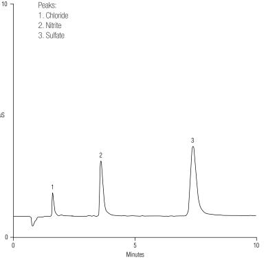
Analysis of simulated rainwater, SRM 2694-II.
