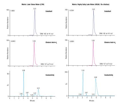
Conductivity and SRM chromatograms of endothall spiked in different samples: left, 5 ppb endothall in salty lake water with 10-fold dilution.
