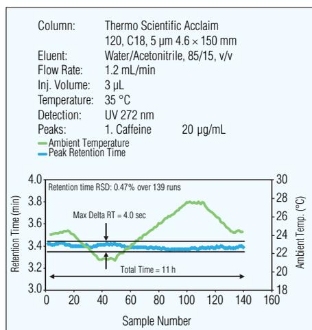
The column compartment of the ACC-3000 allows robust peak identification by retention time, even at fluctuating ambient conditions.
