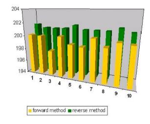
Figure 3: Pipetting results with glycerol using the forward method and the reverse method. The pipette was adjusted for glycerol using the forward method.
