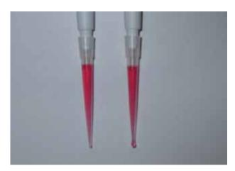
Figure 2: Evaporation causes the liquid to squeeze through the tip orifice if the tip is not pre-wetted. On the right a dry tip, and on the left a pre-wetted tip with a colored ethanol solution 15 s after the aspiration.
