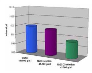
Figure 1: Effect of liquid density on the delivery volume. Differences between water, saturated NaCl solution and 20 w-% Na2CO3 solution. Individual measurement variation shown along with the average value of test results.
