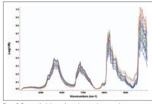
Figure 6: Spectra of ethylene-polypropylene copolymer samples. Concentration of polyethylene ranged from 2% to 16%.
