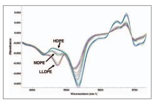
Figure 3: First derivative spectral range analyzed for discriminant analysis of the different polyethylene density classes.
