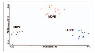
Figure 4: Principal component scores plot demonstrating clear spectral separation between the different density classes of polyethylene.
