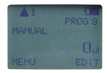
The large screen displays aspirated or dispensed volume and speed for continuous control of pipetting action.
