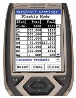
Users can set limits for pass/fail thresholds. For example, Br+Cl is set to 1500 +/- 200 ppm in plastics mode.
