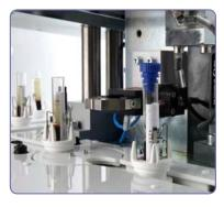
Recapper Module – Automatic capping of different types and sizes of primary and TCAutomation Aliquoter secondary tubes with conical caps.
