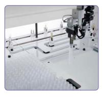
Aliquoter/Labeler Module — Automatic sample aliquoting to secondary tubes using disposable tips. Automatic barcode labeling of secondary tubes.
