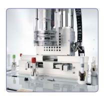
Decapper Flex Module — Automatic cap removal from different types and sizes of sample tubes.
