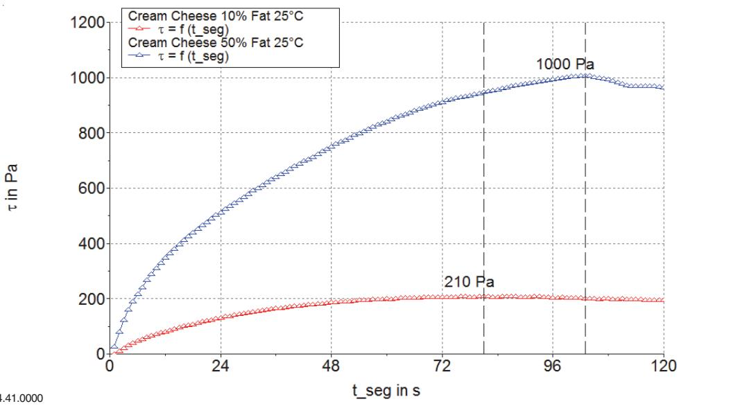
Fig. 2: Shear Stress versus Time for the two different cream cheese products at 25 °C
