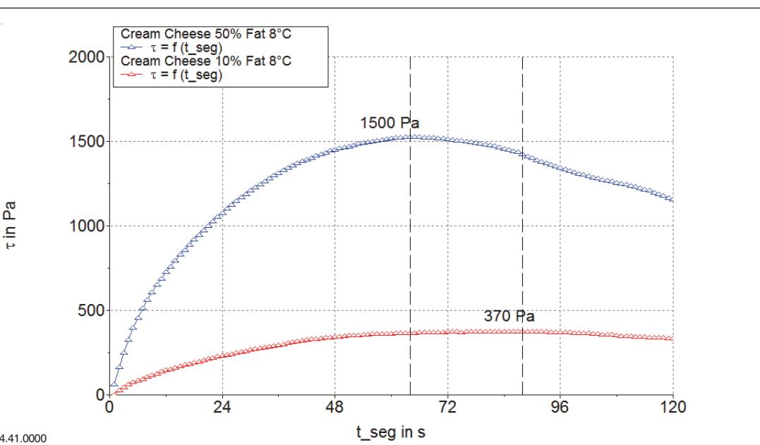
Fig. 3: Shear Stress versus Time for the two different cream cheese products at 8 °C
