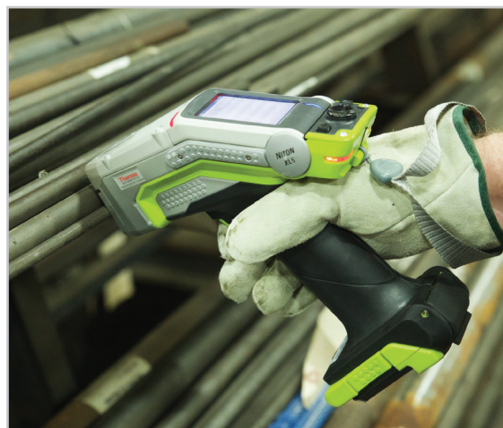
An inspection is conducted using the handheld Thermo Scientific™ Niton™ XL5 XRF analyzer.
