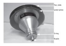
Separate body from impaction chamber
