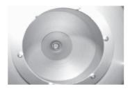
Remove the inlet plates and clean screen Wipe out inside of body
