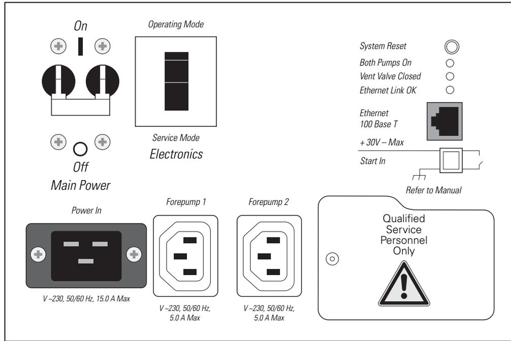
**Figure 35.** Power panel of the TSQ Quantum Access, or TSQ Quantum Access MAX, showing the Main Power circuit breaker switch, Electronics service switch, Vacuum service switch, and System Reset button
