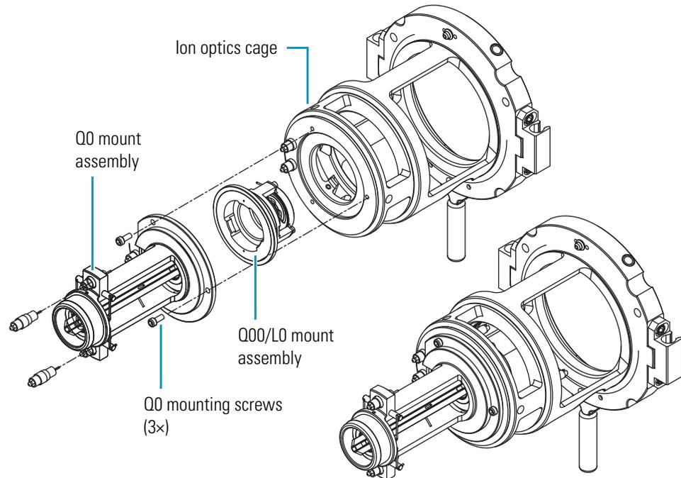
2. Remove the Q0 mount assembly. Place it on a clean, lint-free surface.
