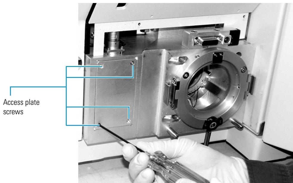
3. Unplug the ion source cable harness from the connector. See [Figure 52](#).
