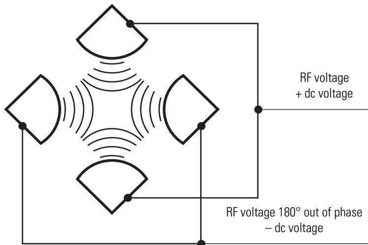
The ac voltage applied to the quadrupole rods is of constant frequency (1.123 MHz). The rf voltage applied to the rods varies from 0 to 10 000 V peak-to-peak, and the dc voltage varies from 0 to  $\pm 840$  V. Voltages of the same amplitude and sign are applied to each rod pair. However, the voltages applied to the other rod pair are equal in amplitude but opposite in sign.
