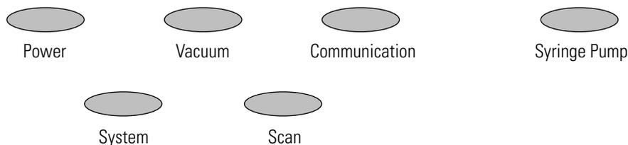
The Power LED illuminates green whenever power is supplied to the vacuum system and electronic assemblies of the mass spectrometer.
