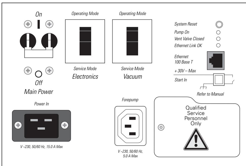
The electronics service switch (labeled Electronics) is located next to the main power circuit breaker on the mass spectrometer power panel (Figure 12 and Figure 13). In the Service Mode position the switch removes power to all components of the mass spectrometer other than the vacuum system. The Operating Mode position supplies power to all non-vacuum system components of the mass spectrometer.
