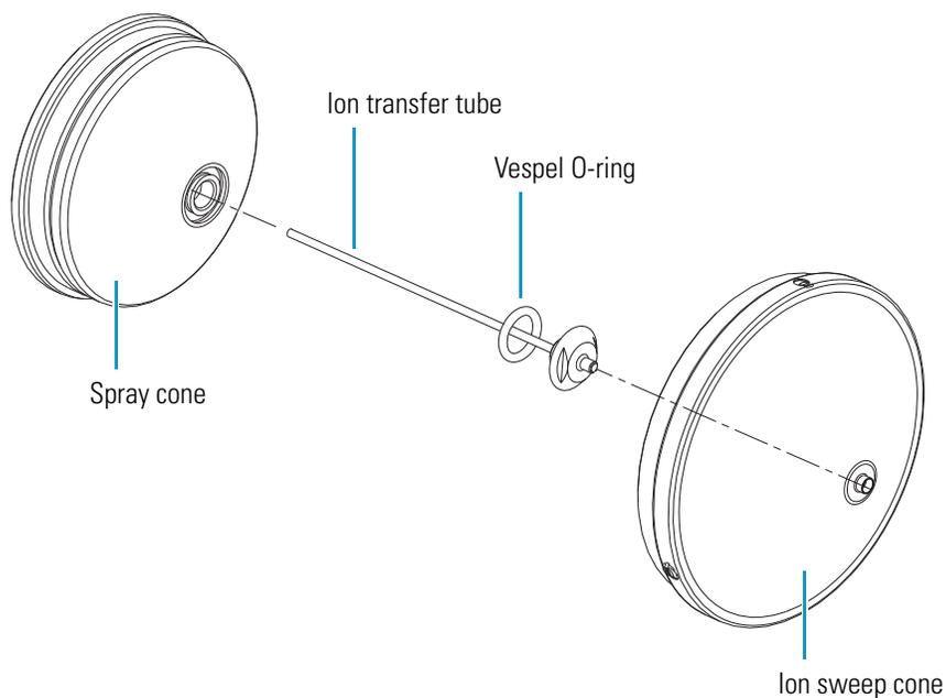
7. Soak the ion transfer tube in a dilute solution of nitric acid to remove contaminants.
