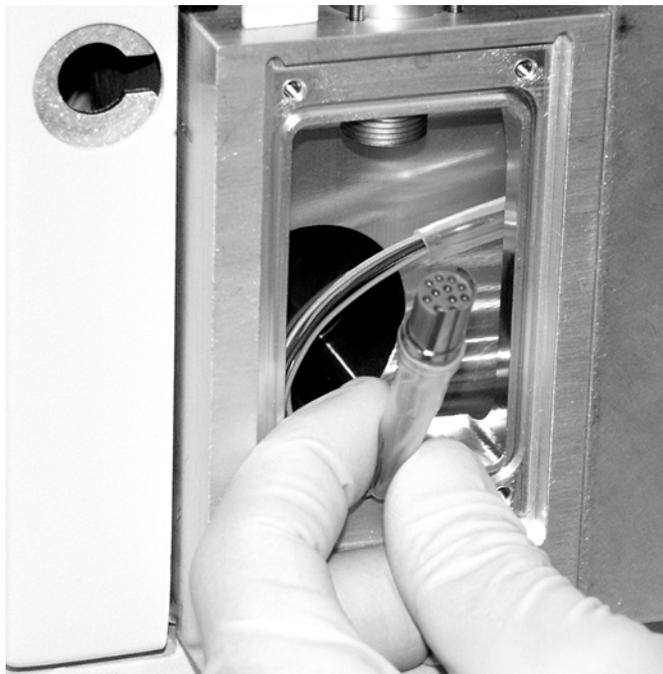
4. Remove the ion optics cage assembly:
