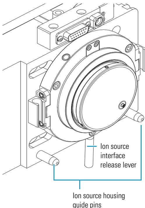
2. Rotate the ion source housing locking levers 90 degrees to lock the ion source housing onto the ion source mount assembly.
