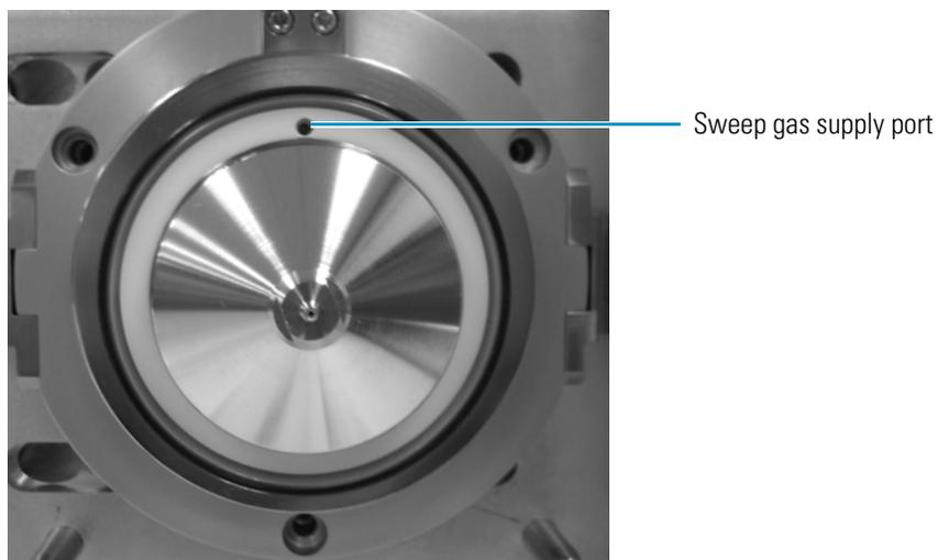
**Figure 45.** Ion sweep cones for FAIMS and APPI (left) and H-ESI, ESI, and APCI (right), showing the gas inlets
