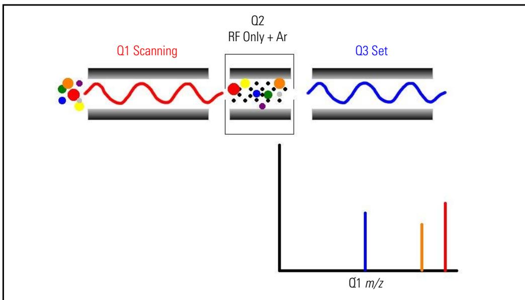
Experiments that employ the parent scan mode (parent experiments) can be used in structure and fragmentation studies as well as in survey analyses of mixtures. In general, parent experiments detect all compounds that decompose to a common fragment. The experiments are useful for the rapid detection of a series of structural homologs (for example, substituted aromatics, phthalates, steroids, or fatty acids) that have a common fragment ion (for example,  $m/z$  149 for the phthalates).
