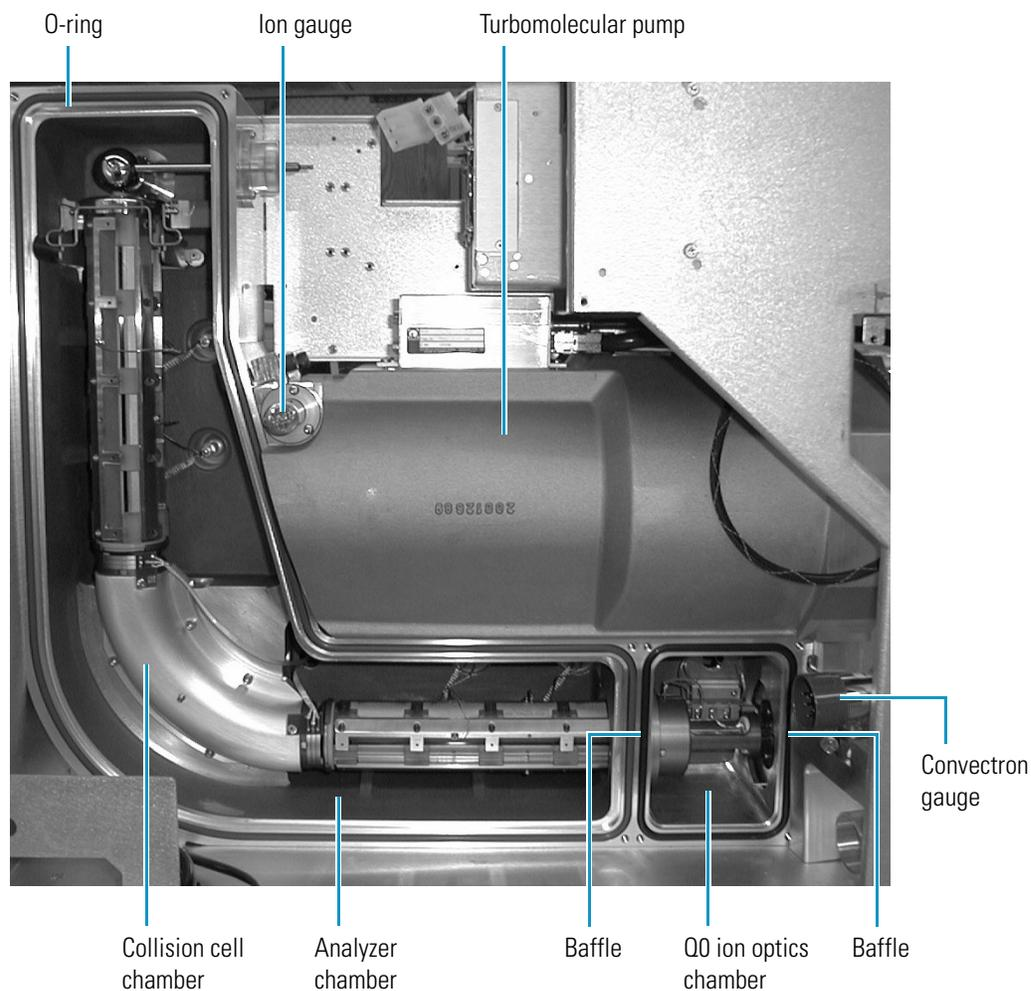
The collision cell chamber, inside the analyzer chamber, has a user controlled argon pressure of between one and four mTorr when CID is turned on. Argon in the collision cell is evacuated by the forepump when CID is turned off.
