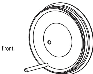
**Figure 19.** Exit lens of the TSQ Vantage
