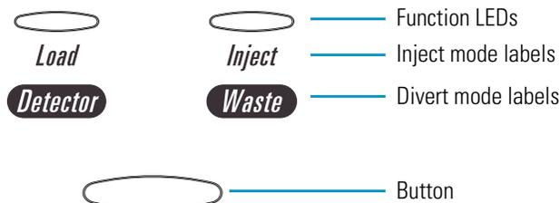
When the divert/inject valve is set up for divert valve operation, the divert/inject valve button switches the LC flow between the mass spectrometer and the waste container and the labels *Detector* and *Waste* apply.
