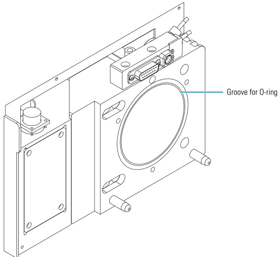
2. Orient the ion optics cage assembly with the contact pins down, and then partially insert it into the ion source mount assembly.
