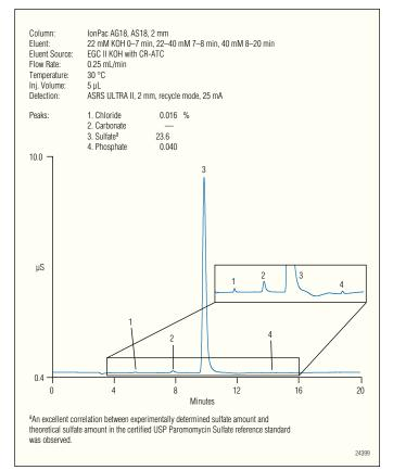
Figure 2. Separation of sulfate counter ion and anionic impurities in USP-grade paromomycin sulfate.
