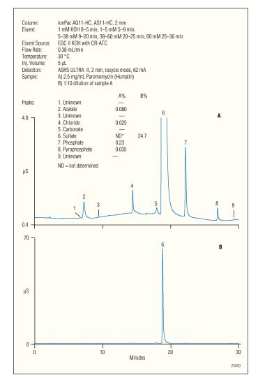
Figure 3. Separation of sulfate counter ion and anionic impurities in Humatin using the IonPac AS11-HC.
