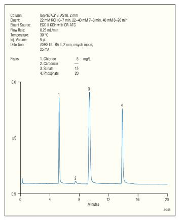
Figure 1. Separation of target anions on the IonPac AS18 column.
