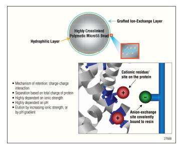
Figure 2. Separation media and mechanism of cation-exchange columns.
