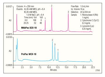
Figure 3. Selectivity differences: MAbPac SCX-10 vs ProPac WCX-10 columns. Ribonuclease A elutes prior to other proteins in MAbPac SCX-10 as compared to ProPac WCX-10 showing a selectivity change. Such orthogonal selectivity differences are quite helpful in protein heterogeneity characterization.
