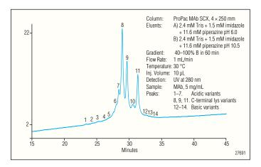
Figure 6. pH gradient-based MAb separation.<sup>3</sup> With the use of a pH gradient, the MAbPac SCX-10 column provides high-resolution separation of monoclonal antibody variants.
