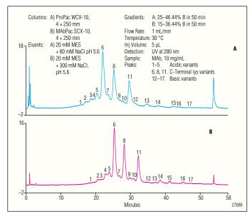
Figure 4. MAb separation: Comparison of ProPac WCX-10 vs MAbPac SCX-10 columns. The ProPac WCX-10 and MAbPac SCX-10 columns provide high resolution and peak efficiencies of monoclonal antibody acidic, basic, and C-terminal lysine variants.
