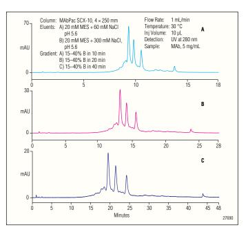
Figure 5. MAb separation on the MAbPac SCX-10 column using different gradients. MAb analysis was achieved under 15 min with high resolution.
