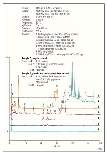
Figure 8. Analysis of Fab and Fc fragments of a MAb after digestion with carboxypeptidase and papain using the MAbPac SCX-10 column.
