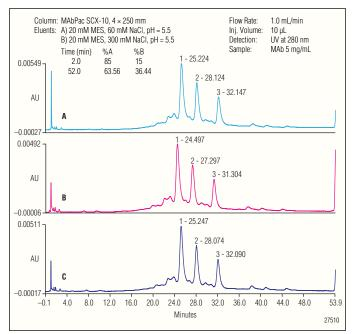
Figure 9. Lot-to-lot reproducibility of the MAbPac SCX-10 column. Columns from each of the three different lots (A, B, C) were used for MAb analysis. Retention times for the C-terminal lysine variants are shown.
