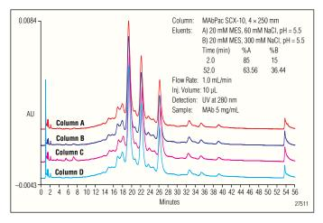
Figure 10. Column-to-column reproducibility of the MAbPac SCX-10 column. No change in performance was noted for 4 different MAbPac SCX-10 columns (A, B, C, D) from the same lot.
