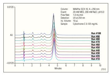
Figure 11. Ruggedness of the MAbPac SCX-10 column. More than 100 isocratic runs were performed to assess the reproducibility, ruggedness, and column performance. The chromatography profiles remain unchanged.
